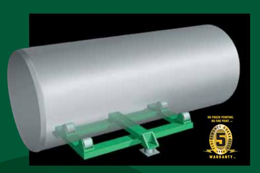
TODAY, AFTER MORE THAN 30 YEARS, THE HYDRAULIC CHLOR-SCALE® CONTINUES TO BE THE MOST DURABLE AND RELIABLE SYSTEM AVAILABLE FOR MONITORING TON CONTAINERS OF CHLORINE AND SO2. SCALE FRAMES ARE BUILT OF HEAVY-DUTY GRADE ASTM A36 STEEL AND THEN COATED WITH OUR 2-PART EPOXY FINISH. ZINC PLATED STEEL ROLLER TRUNNIONS SAFELY CRADLE THE CONTAINER AND ALLOW EASY ROTATION OF THE TANK FOR CORRECT VALVE POSITIONING.
